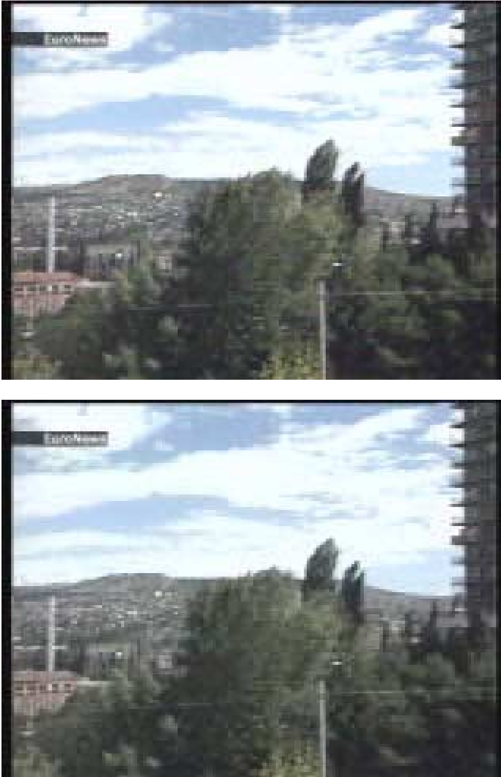
Fig. 12. Sample reconstructions. Top: an original frame from a GOP with a significant amount of motion (the camera is panning over a relatively complex scene, with rich textures); bottom: a frame from the GOP reconstructed by 1cavpc35 in 0.6 seconds. The PSNR for this GOP is 33 dB—in real-time playback, it is impossible to tell the difference between the original frame and the reconstructed one.
