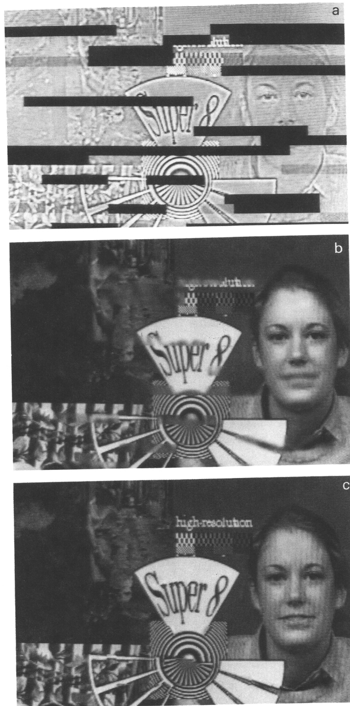
Fig. 5. Effect of error concealment for 15% fine-channel packet loss (blow up of Fig. 4). (a) Corrupted spatial residual frame. (b) Reconstruction without error concealment. (c) Reconstruction with error concealment.
