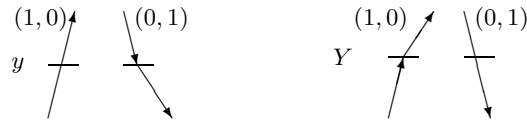
Fig. 4.6. Sketch of the possible sample paths crossing the buffer levels y (left) and Y (right) in case v_1^+ = v_2^+ . The slope of the arrows are proportional to v_1 - v_2 . In the stationary regime, the upward flow equals the downward flow.
