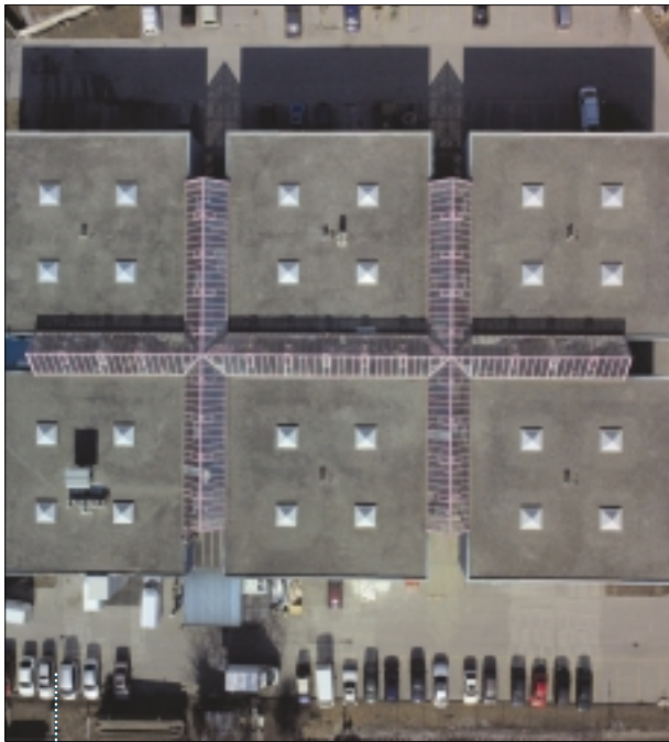
Figure 4 - HELIMAP mapping results. Left: high resolution ortho-rectified image. Right: high resolution digital surface model with point density of 0.2m and accuracy of 0.05–0.15m.
