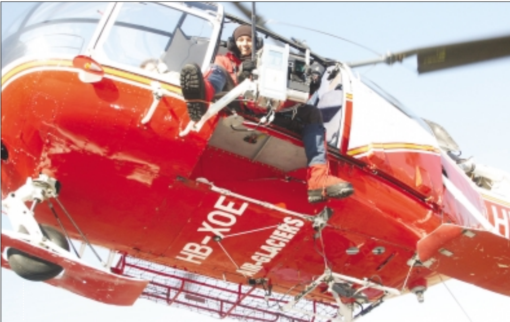
Figure 3 - HELMAP: Handheld mobile mapping system on a helicopter integrating GPS/INS with high-resolution CCD digital camera and Airborne Laser Scanner (ALS).
