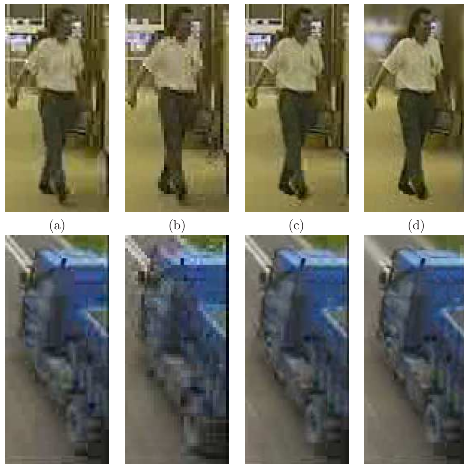
Figure 6.16: Details of frame 280 of Hall monitor (top) and frame 16 of Highway (bottom). The sequences are encoded with MPEG-1 at 150 Kbit/s using different adaptation strategies. (a) Coded original sequence. (b) Spatial resolution reduction. (c) Static background. (d) Lowpass-filtered background.
