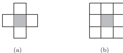
Figure 2.3: Pixel adjacency describes the neighborhoods of a pixel. (a) 4-neighbors. (b) 8-neighbors of the central pixel.
