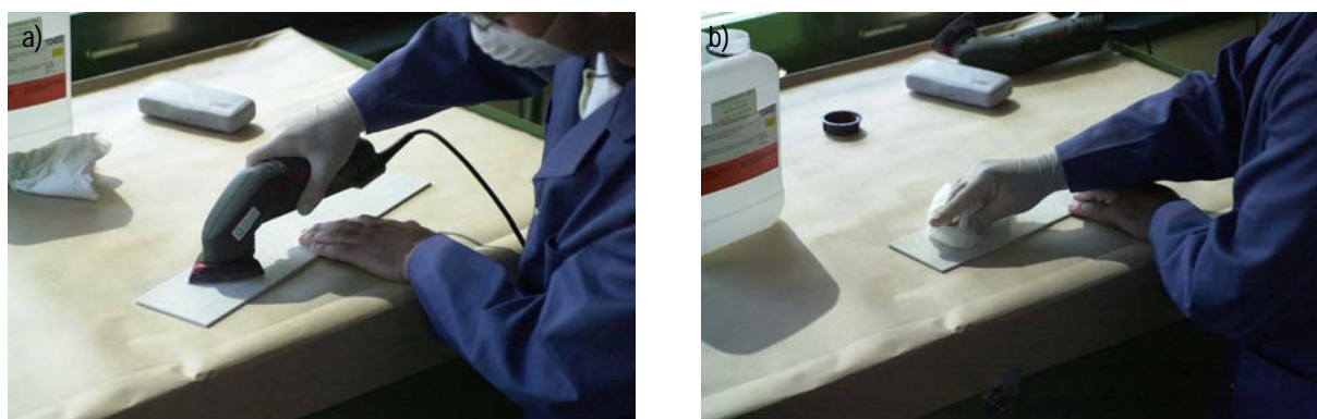
Figure 10 Surface treatment (a) sanding and (b) degreasing
