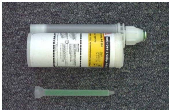
Figure 8 ADP (SikaFast 5221) in a cartridge (250 ml), used for small series, and the appropriate static mixer tube
