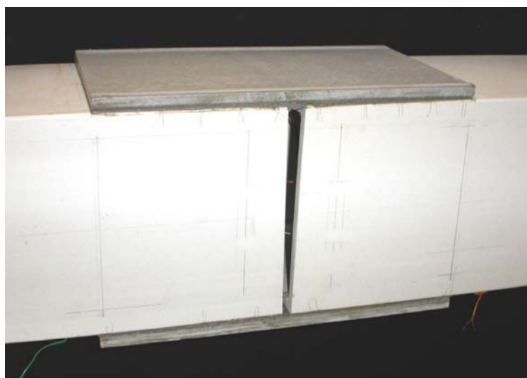
Figure 12 Adhesively-bonded connection of beam PH2
