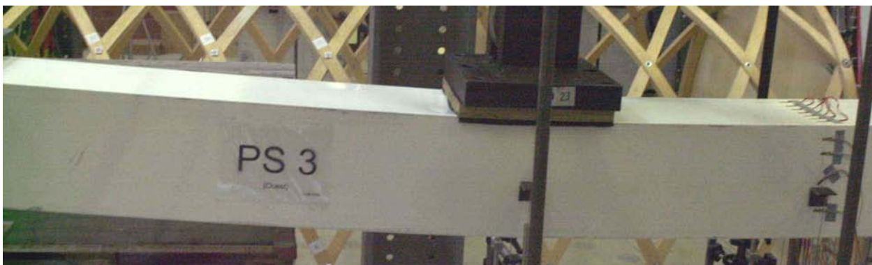
Figure 29 Buckling deformation in beam PS3
