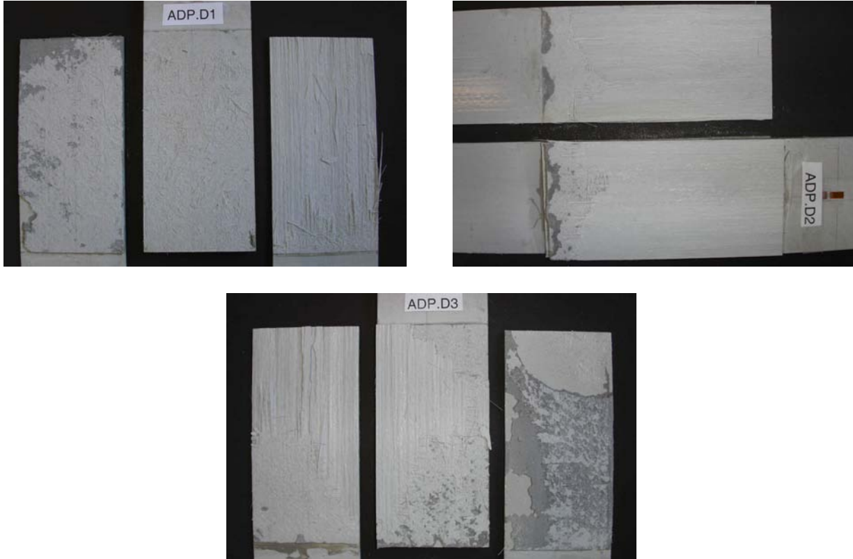
Figure 82 Failure of specimens ADP.D
