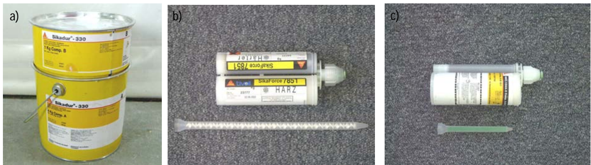
Figure 8 (a) EP (SD 330); (b) PU (S-Force 7851) and (c) ADP (SikaFast 5221) in a cartridge container useful for small series (215 ml and 250 ml), and the appropriate static mixer tube
