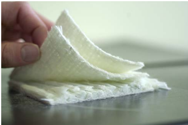
Figure 5 10 mm GFRP laminate (a) fiber architecture after matrix burn-off (without surface veil), (b) microscopic section through thickness: rovings in centre, mats on outside (Tirelli 2003)
