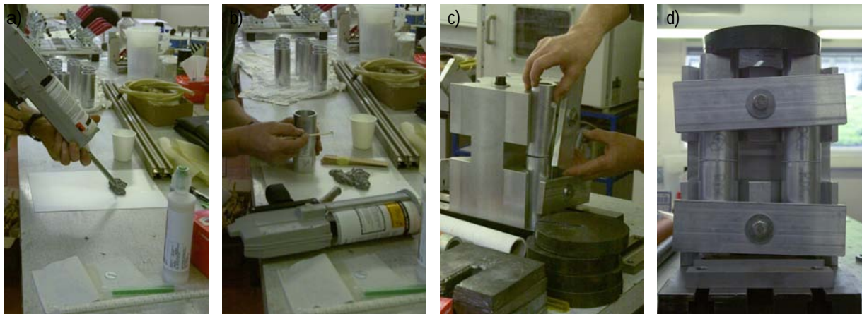
Figure 29 Specimen manufacture: (a) adhesive preparation; (b) adhesive applied to bottom cylinder; (c) cylinder bonding; (d) specimen cure
