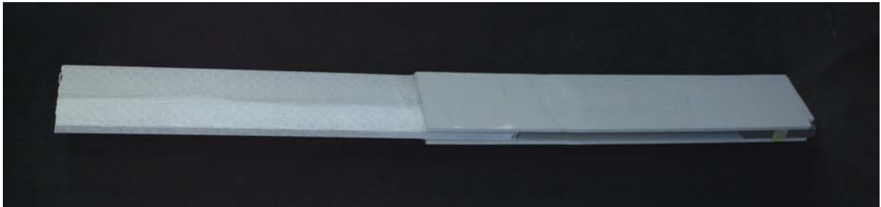
Figure 1 Adhesively-bonded double-lap joint
