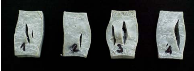
Figure 25 ADP compression specimens after failure
