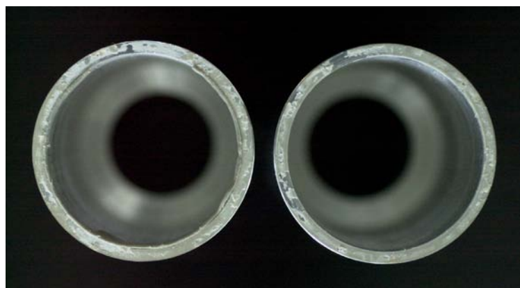
Figure 36 ADP shear specimen after failure
