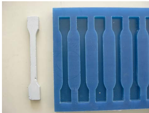
Figure 8 Specimen 1A manufactured using a cast mold
