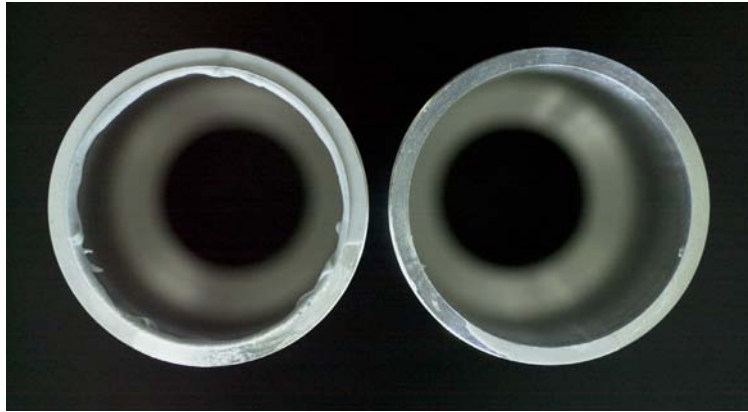
Figure 34 EP shear specimen after failure
