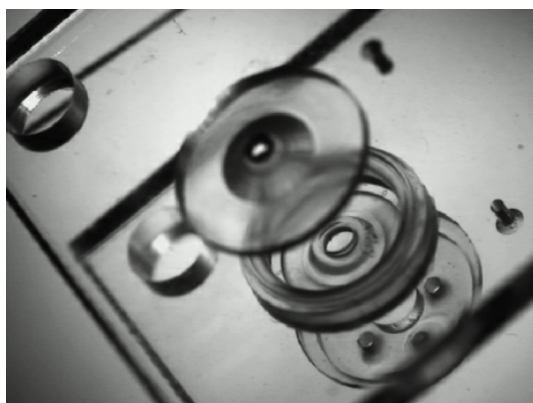
Figure 5-5: Burst view of a silicone membrane check-valve before assembly between two micromachined PMMA plates.
