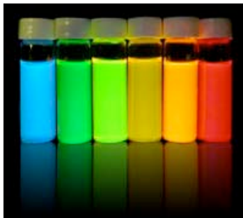
Figure 1.1.1: Fluorescence photograph of solutions containing CdSe nanocrystals of different sizes, from blue the smallest to red the biggest ones. This illustrates well the variation of the emitting domains with increasing sizes. This image is taken from the Biopixel website.
