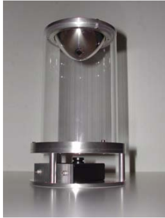
Figure 2.9: The SOLERO omnica. The shape of the mirror is specified by the equation. For this design, the parameters r_0 and \alpha are respectively 14 cm and 11^\circ .
