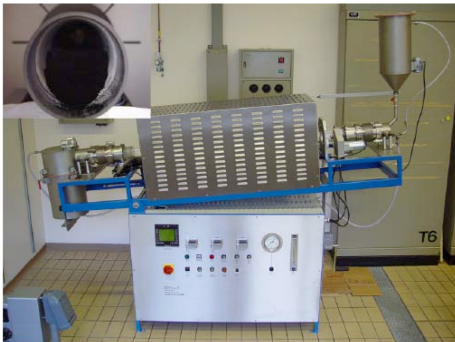
Fig. 2.2: View of the rotary-tube oven used for large-scale synthesis of CVD nanotubes. Two reservoirs are located at the ends of the tube, one containing the catalyst (right-hand side) and the other collecting the product (left-hand side).
