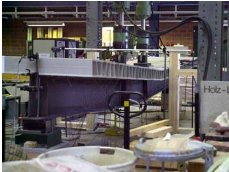
Figure E.29: Side view from right with large deformations at the onset of failure
