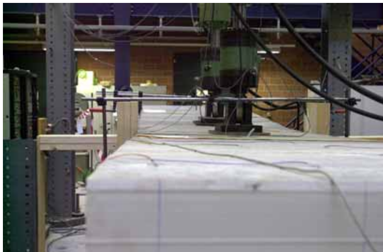
Figure E.24: Side view from right with visible large deflection at \sim 280 kN/jack
