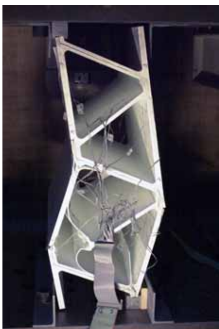
Figure C.5: Failure pattern AS-1
