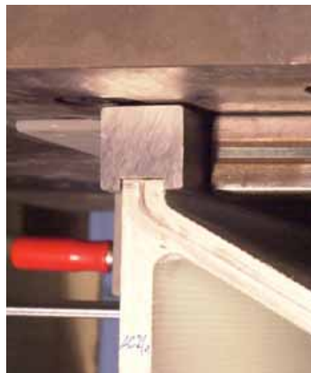
Figure 3.14: Force-introduction point with load-application device for ASSET specimens
