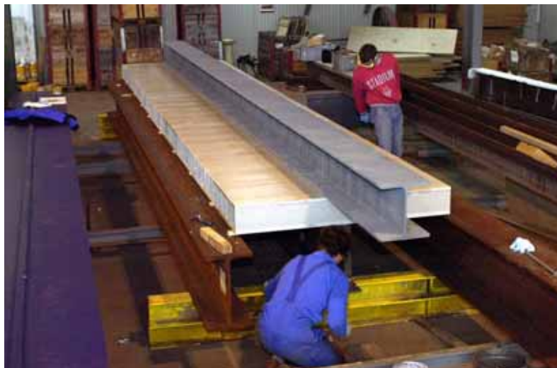
Figure 4.12: Girder Fix 1 with weight after bonding
