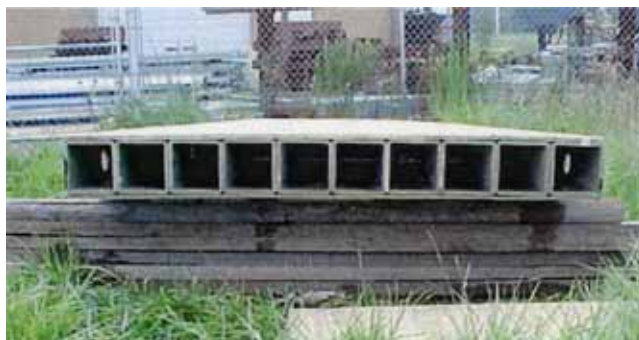
Figure 2.8: End view of Virginia Tech Deck
