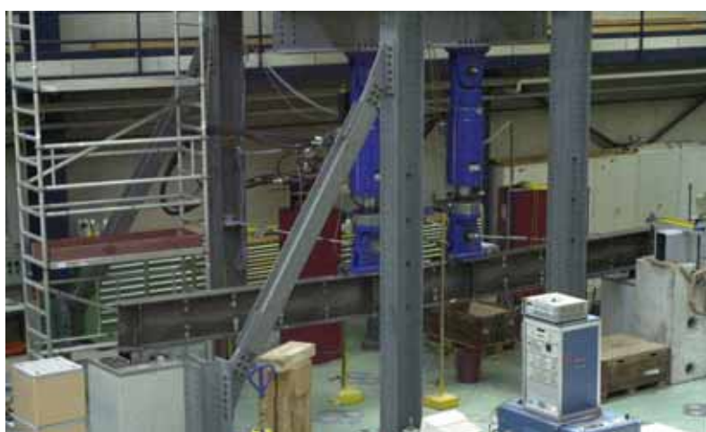
Figure E.1: Set-up of steel-girder experiment - overview
