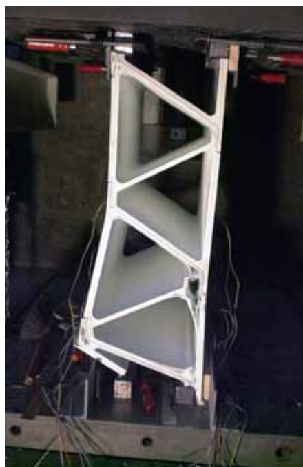
Figure C.4: Failure pattern AC-4
