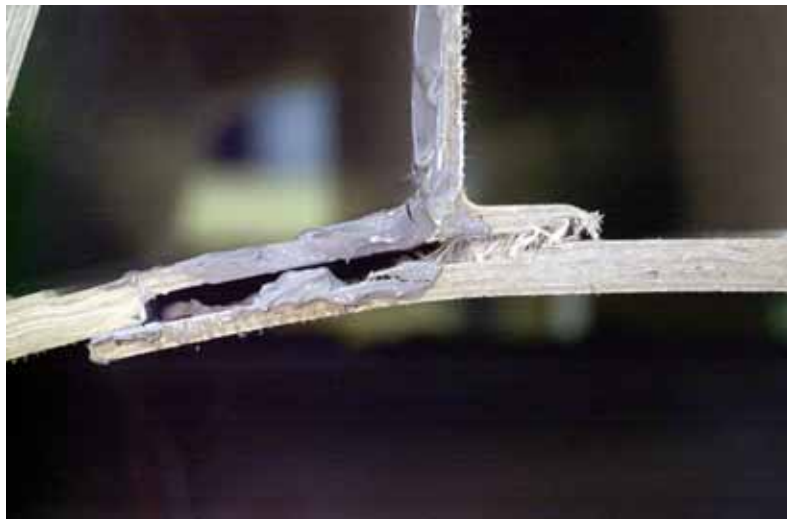
Figure E.32: Same axis as in Fig. E.31 but lower face sheet. Combined compression/shear failure
