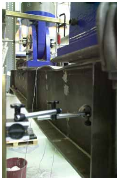
Figure E.4: Buckling of upper steel flange (left side)
