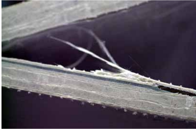
Figure E.33: Detail of a polyurethane joint with failure in the first layer of the FRP (the adhesive joint stays intact)
