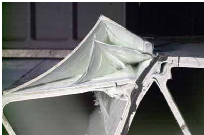
Figure E.7: Location of first failure (Axis G - G) after end of experiment with large delamination
