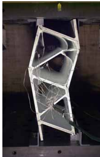
Figure 3.40: Failure pattern, specimen AS3
