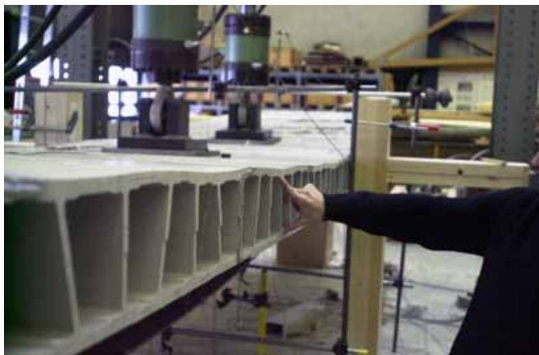
Figure E.27: Undulated deformation of the upper face sheet due to Vierendeel action (at the onset of failure)
