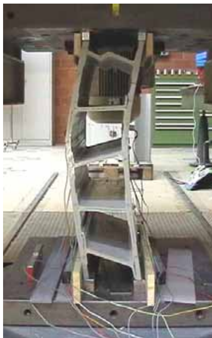
Figure 3.21: Typical failure pattern of compression experiments (Specimen 3as)
