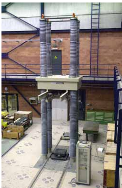
Figure 3.8: Trebel 10,000-kN press
