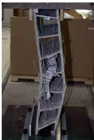
Figure 3.37: Failure pattern, specimen 4as
