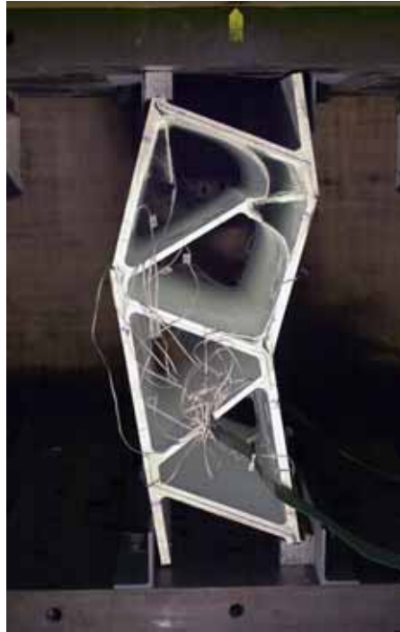
Figure C.7: Failure pattern AS-3
