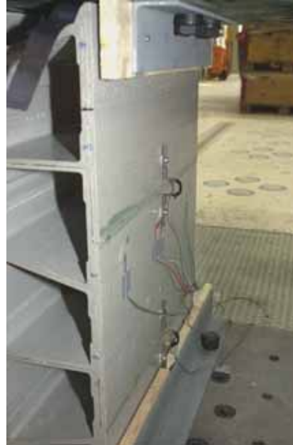
Figure 3.9: Installed \Omega -gages on DuraSpan specimen
