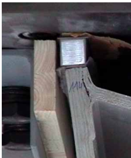
Figure 3.13: Force-introduction point with load-distributing steel sheets for DuraSpan specimens
