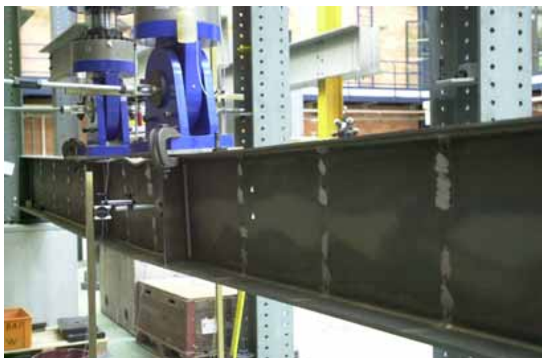
Figure E.2: Buckling of upper steel flange (left side)
