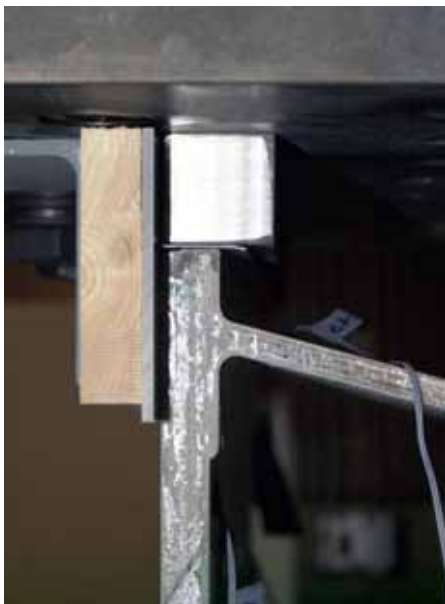
Figure 3.19: Force introduction point with load-distributing steel sheets
