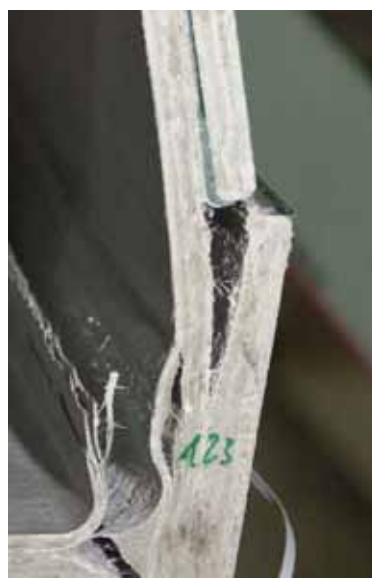
Figure 3.38: Failure pattern, specimen 4as; detail adhesively-bonded joint
