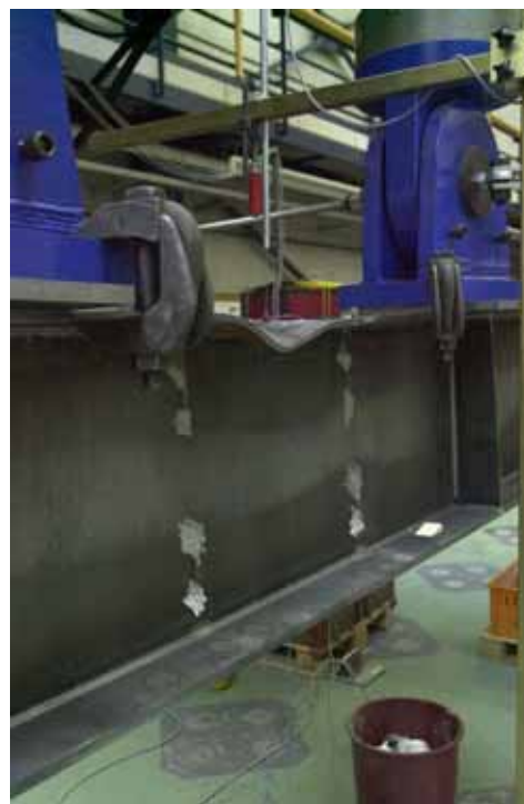
Figure E.5: Buckling of upper steel flange (right side)
