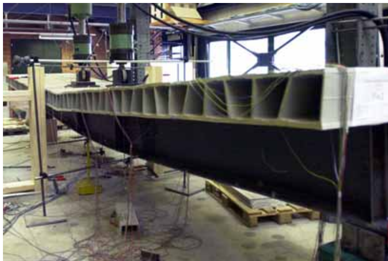
Figure 4.51: Deflection of girder Fix 2 at onset of failure, undulated deformation of upper face panel due to Vierendeel action.
