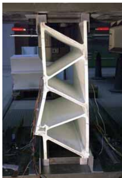
Figure 3.27: Failure pattern of specimen AC2
