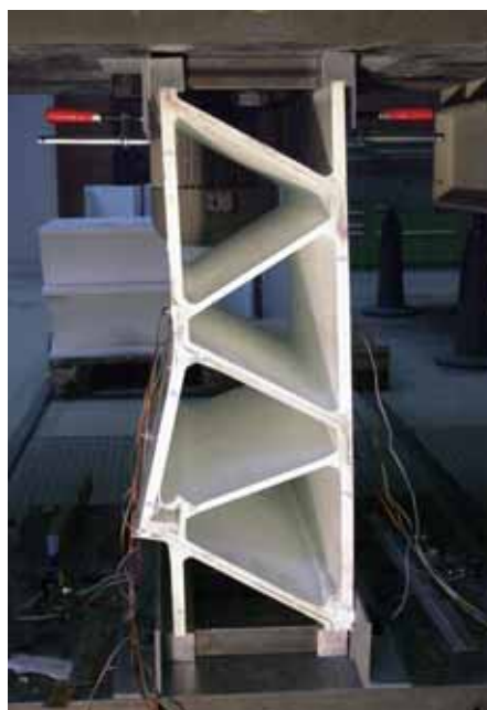
Figure C.2: Failure pattern AC-2
