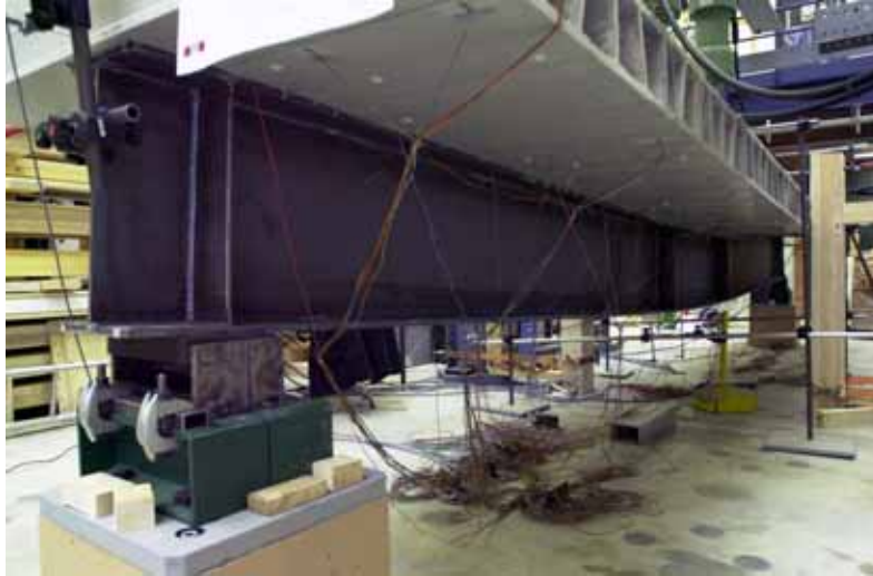
Figure E.25: Bottom view with large deflection and plastic hinges under the jacks
