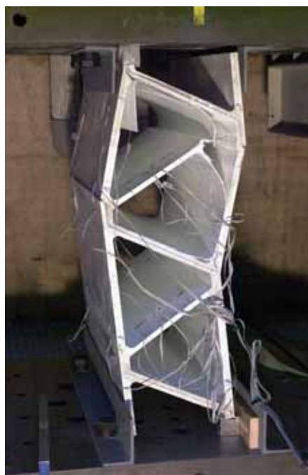
Figure C.6: Failure pattern AS-2
