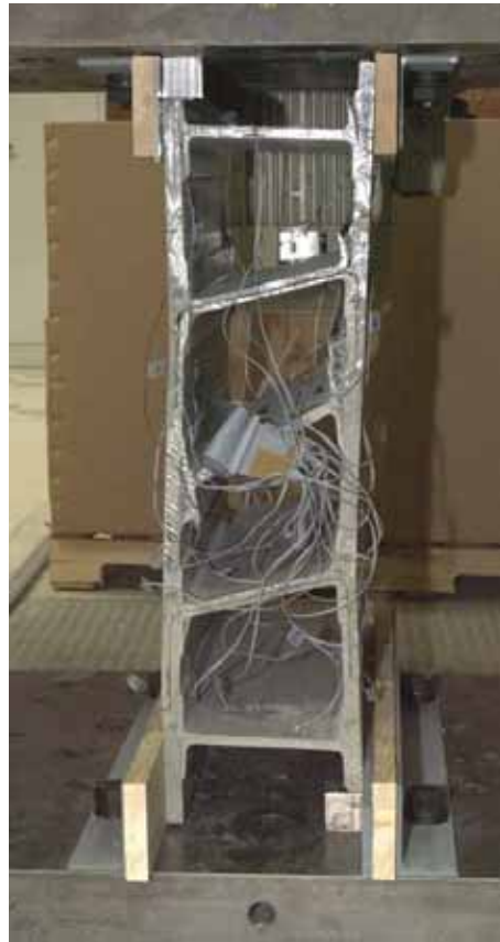
Figure 3.33: Typical failure of three-element specimen (3aa)
