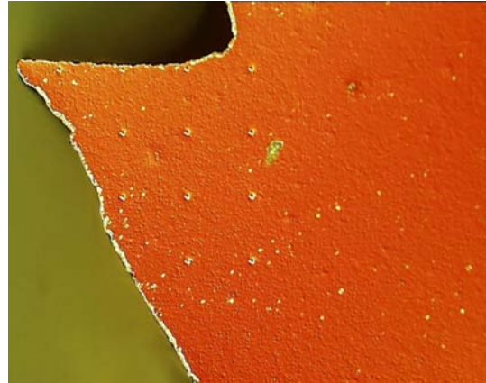
FIGURE 3.26. Placing of the indents on the file tooth. The distance between the indents is 75\ \mu\text{m} and the indentation depth 1\ \mu\text{m} .
