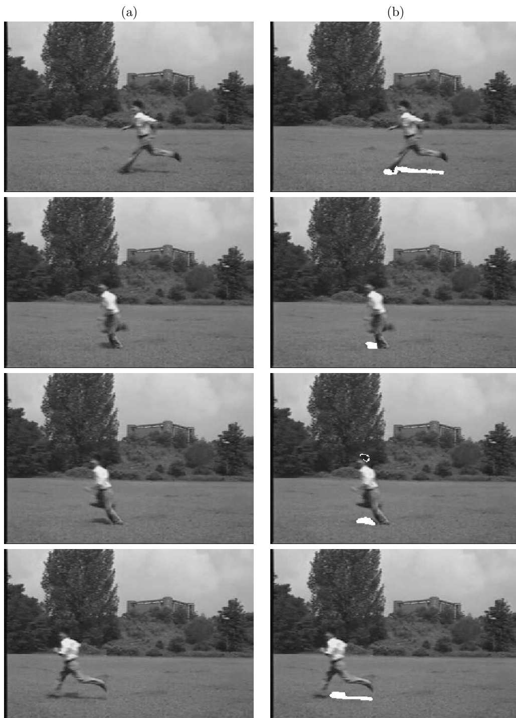
Figure 6.4: Shadow segmentation results for the test sequence Surveillance . (a) Original image; (b) shadow mask (white pixels) superimposed on the original image.
