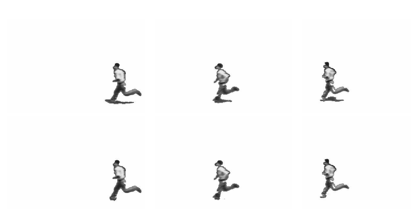
Figure 7.3: Object segmentation results for some sample frames of the test sequence Surveillance without shadow segmentation (first row) and with shadow segmentation and elimination (second row).
