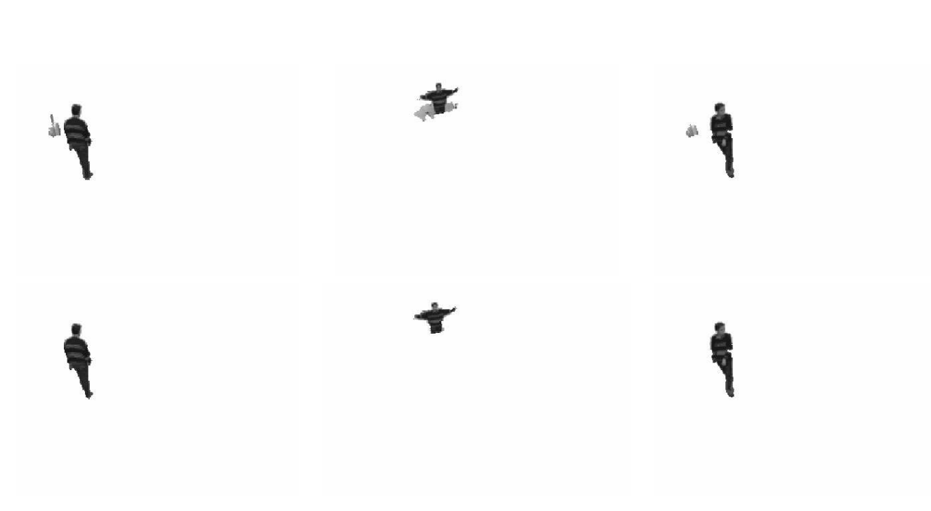
Figure 7.2: Object segmentation results for some sample frames of the test sequence Intelligent room without shadow segmentation (first row) and with shadow segmentation and elimination (second row).
