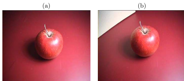
Figure 3.7: Example of inter-reflection in a real image. In (b) a white object is casting light on the observed object.
