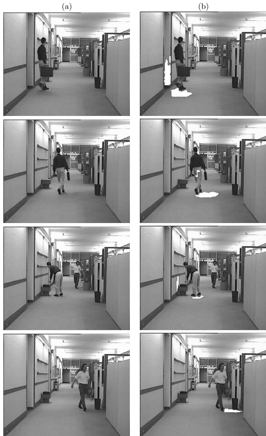
Figure 6.1: Shadow segmentation results for the test sequence Hall Monitor . (a) Original image; (b) shadow mask (white pixels) superimposed on the original image.
