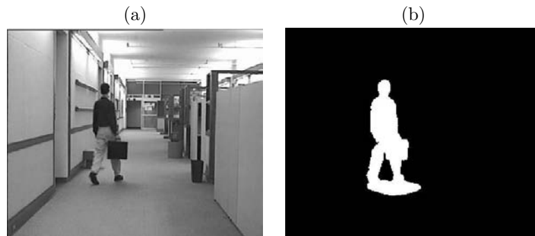
Figure 5.28: Example of change detection results. (a) Original image and (b) change detection mask. White pixels indicate changed areas.
