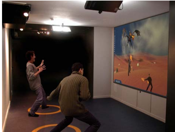
Figure 7.9: Example of immersive interactive mixed-reality environment based on the Magic Mirror metaphor (courtesy of alterface ). The persons in the field of view of the cameras get themselves immersed within the virtual environment and are offered to interact with the story.
