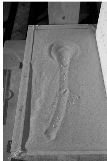
Figure 3.6: Example for a deflection of the rolling trace left by a block.
