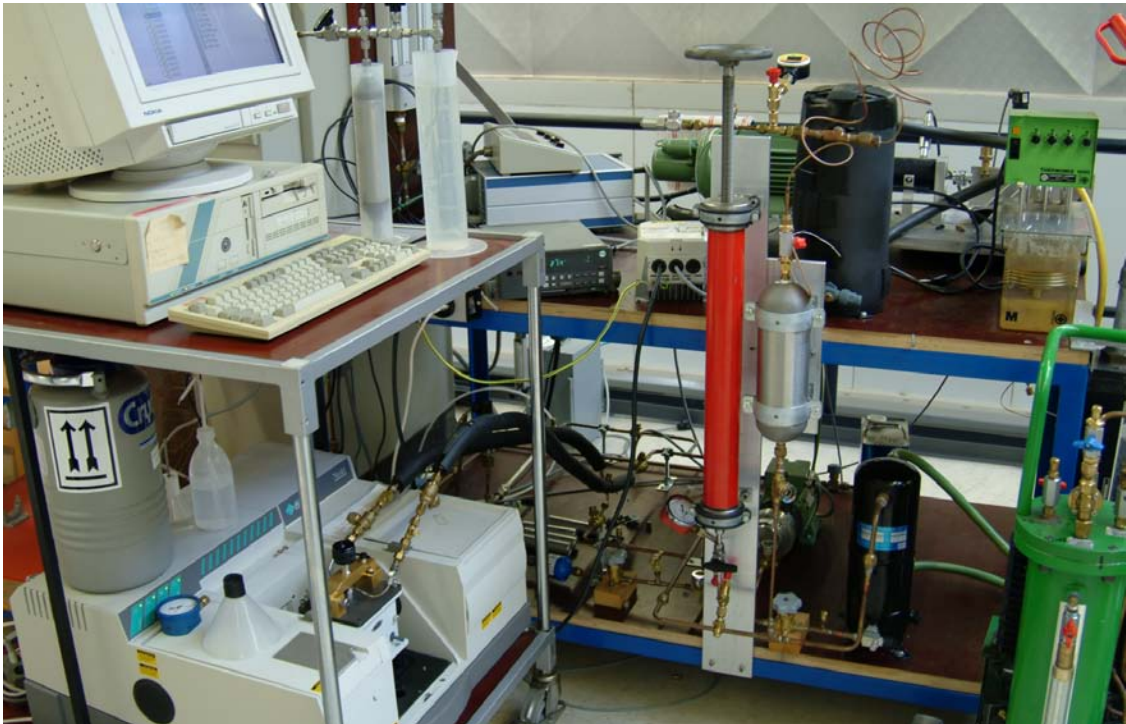
Figure 5.2: Oil concentration calibration test circuit with FT-IR Spectrometer on the left side, oil injection syringe in the center and the liquid refrigerant lines in the lower part of the picture.
