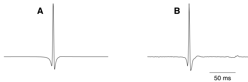
Figure 7.3 — Comparison of simulated and clinical bipolar electrograms, both during sinus rhythm. (A) Simulated bipolar electrogram (normalized amplitude) measured in the right atrium. (B) Clinical bipolar electrogram (normalized amplitude) measured during routine intracardiac mapping. In both case, the distance between the unipolar electrodes is 2 mm.
