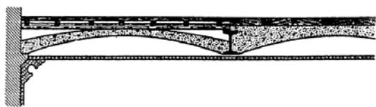
Fig. 20: Cast-iron beam floor bearing system with shallow masonry or concrete vault supported by bottom flange of beam. Shown: Dennett's arch floor. (Sutherland)
