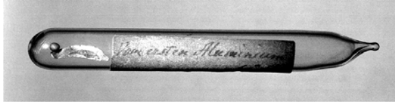
Fig. 12: Test tube holding aluminum particles reduced by Friedrich Wöhler, 1845. (Nichols)
