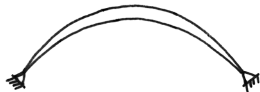
Fig. 3.4: Schematic of a two-hinge arch. (Dooley)
