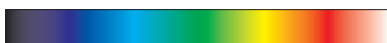
FIGURE 4.1: (Color) Color scale used to display two-dimensional intensity distributions. The color varies in a black-blue-cyan-green-yellow-red-white sequence from low to high intensities.
