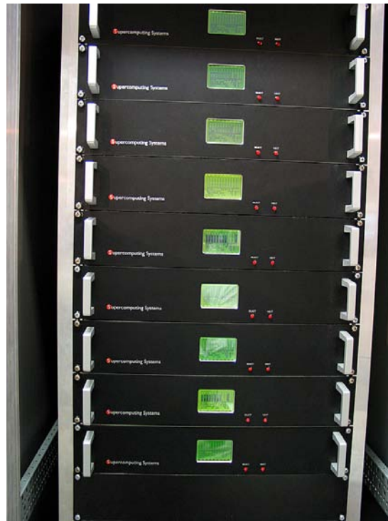
Figure 3.7: The TNet switches with 12 ports each
