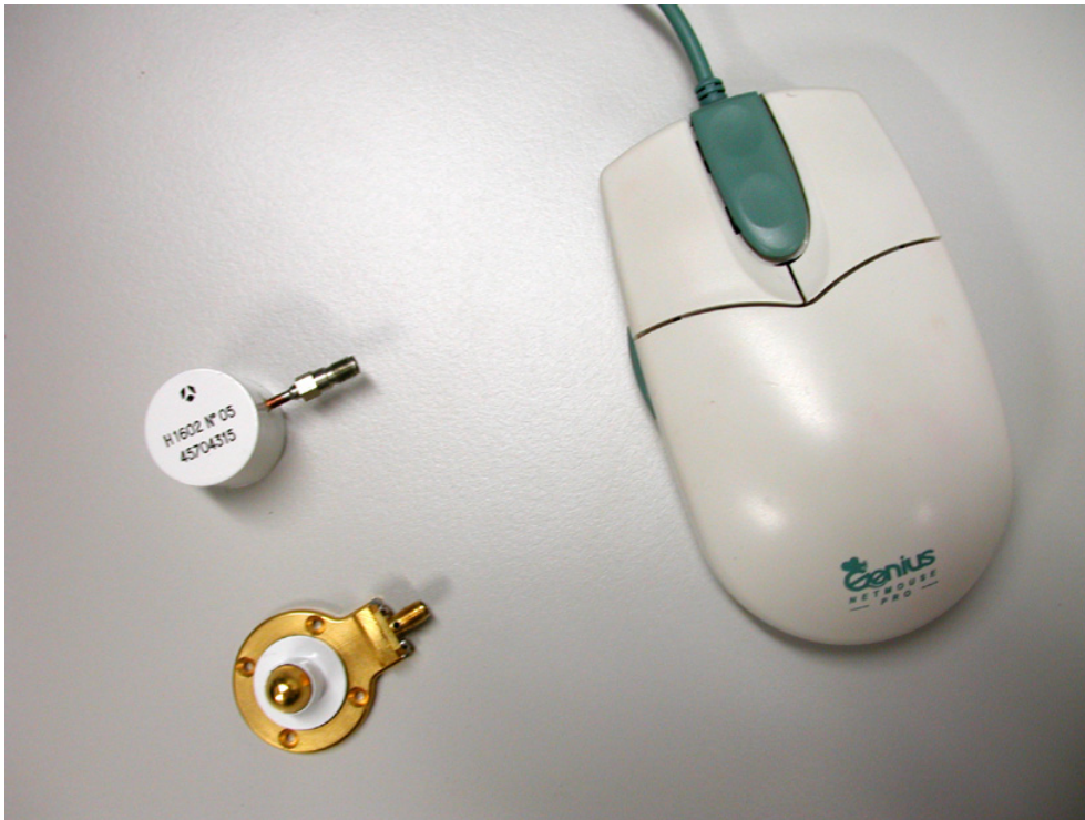
Figure 4.7: Thomson Electric and Magnetic Field Sensors used for the EMP simulator measurements
