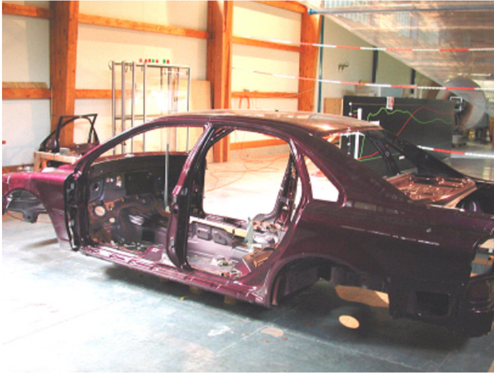
Figure 4.8: Test car inside the simulator (side illumination)
