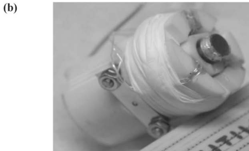
Figure 4.11: (a) Schematic drawing of the scan head of the microscope. This mechanism controls the approach-withdraw movement of the tip and the scan movement of the tip on the surface. The sample holder is also shown. (b) Photo of the scan head of the microscope. The z-piezo is completely up.
