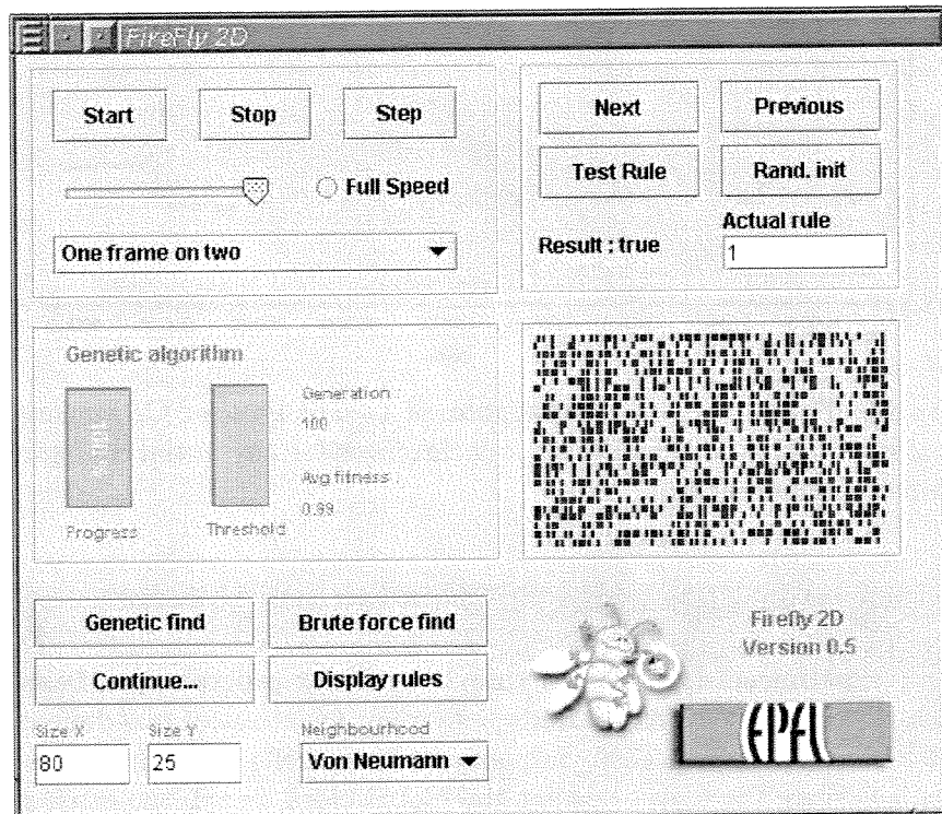
Figure 3.7: The firefly Java program allows to find a solution to the synchronization task by means a co-evolving genetic algorithm. An exhaustive (“brute force”) search can also be performed.
