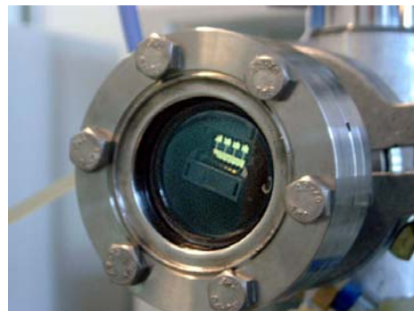
Fig. 26 Window of the vacuum system used for the measurements under controlled atmosphere. Inside, the chip holder holding an I-Plan chip can be seen. During experiments, the chip was observed with a microscope.
