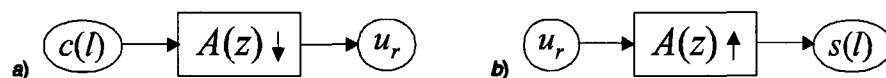
Figure 3.15: Graphic symbols for a) switched dispersive delay lines and b) tapped dispersive delay lines.
