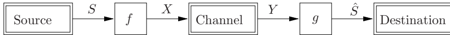
Figure 2.2: The symbol-by-symbol communication system: f : \mathcal{S} \rightarrow \mathcal{X}, g : \mathcal{Y} \rightarrow \hat{\mathcal{S}} .
