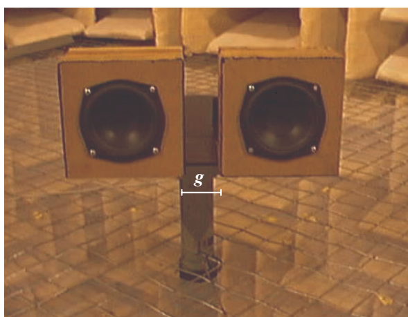
Figure 4.36 - Picture of two closed-box loudspeakers mounted on an immovable stand and separated by a distance g
