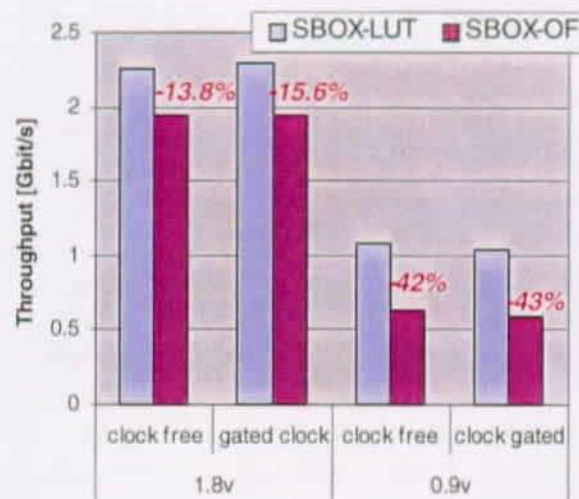
Figure 7-81: Throughput of both SBOX-LUT and SBOX-OF architectures in iterative looping configuration
