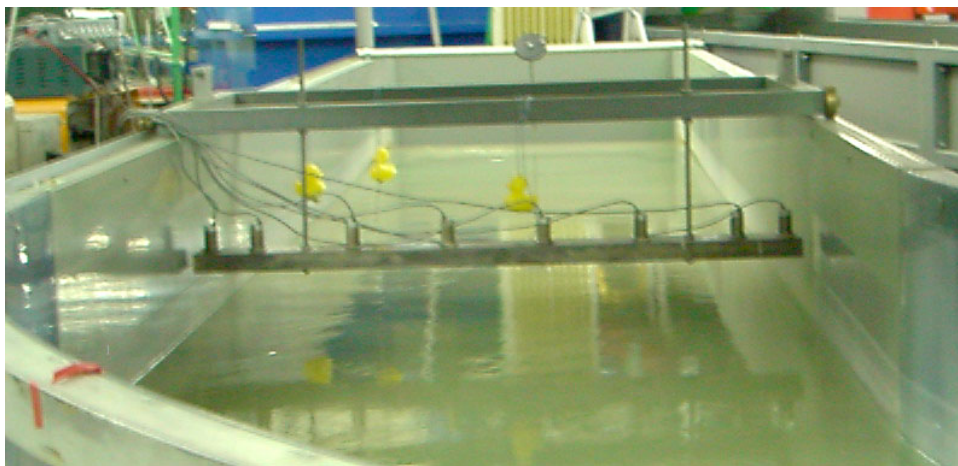
Fig. I.5: Acoustic limnimeters for measuring water-surface and bottom topography
