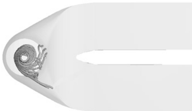
Figure 2.19: Vortex core identified with the eigenvector method of Sujudi and Haines [SH95]. 15 phases equally spaced over a period.
