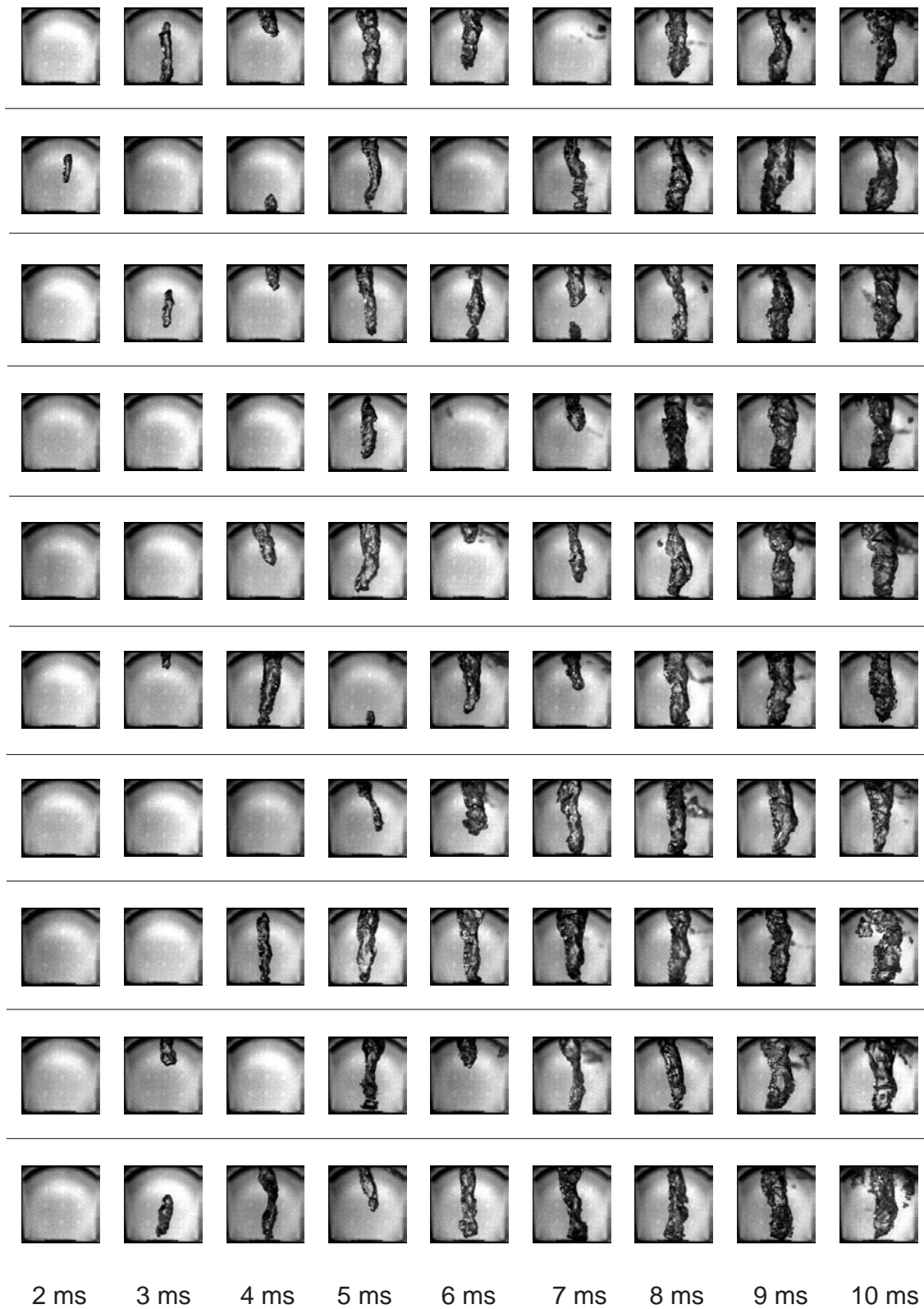
Figure 8.11: Images of cavitation vortex from different time intervals after the valve closure, N=200 \text{ rpm} , Q=0.66 \text{ l/s} , \sigma=1.2
