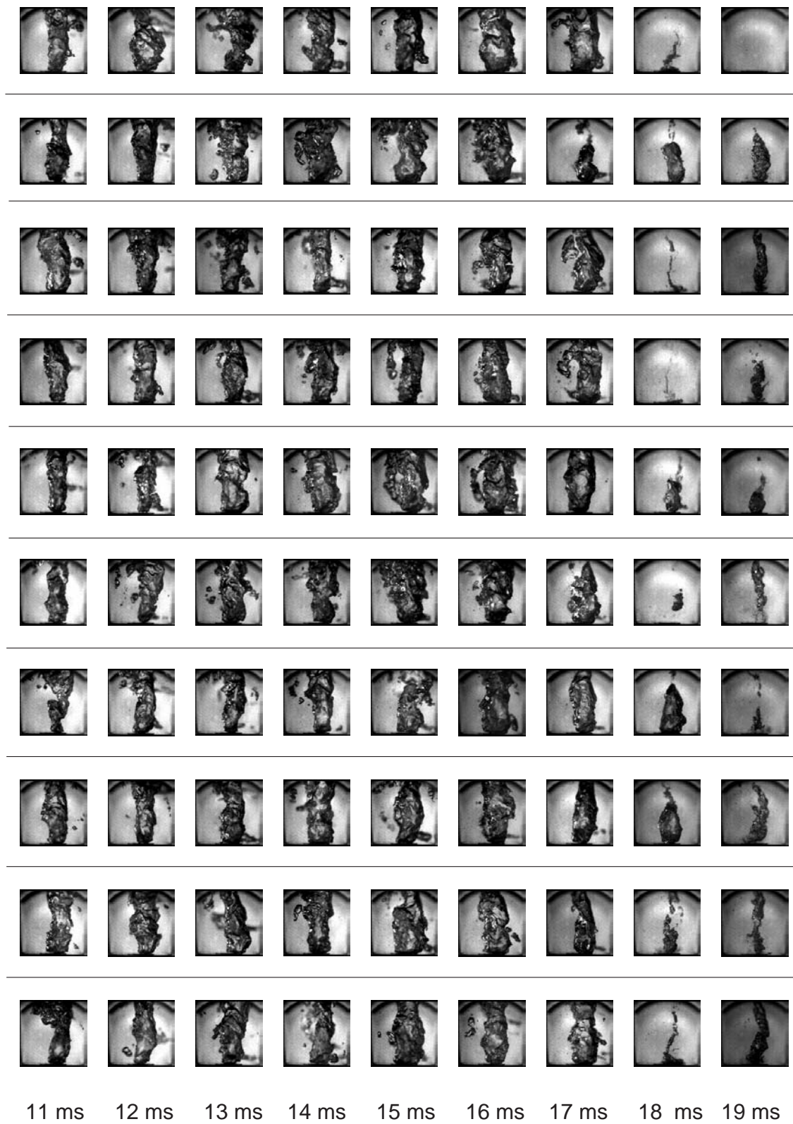
Figure 8.12: Images of cavitation vortex from different time intervals after the valve closure, N=200 rpm, Q=0.66 l/s, \sigma=1.2
