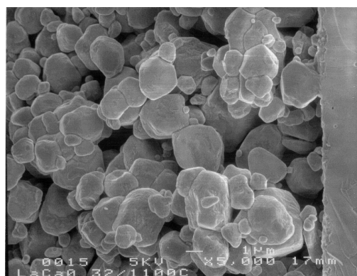
Figure 10: SEM micrographs of the \text{La}_{0.7}\text{Ca}_{0.32}\text{CrO}_3 electrode YSZ electrolyte structure. a: cross-section of the cell showing the topotactic layer; b: the reaction layer surface after removal of the electrode.
