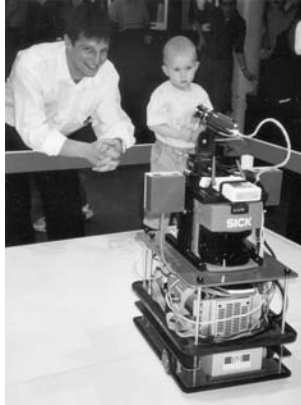
Figure B.2: Daffy Duck, the youngest of our robots, after detecting a young visitor interacts with him by speaking, tracking him and moving the pan-tilt head for mimicking expressions. It detects human movement by means of the CCD camera and closes the interaction loop with its speech synthesizer and gestures as a combination of robot and pan-tilt movement.
