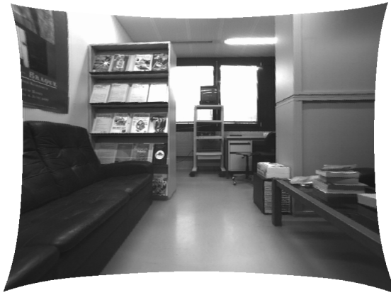
Figure 2.5: A room of the Institute. The image loses its rectangular layout because it is compensated against radial distortion.
