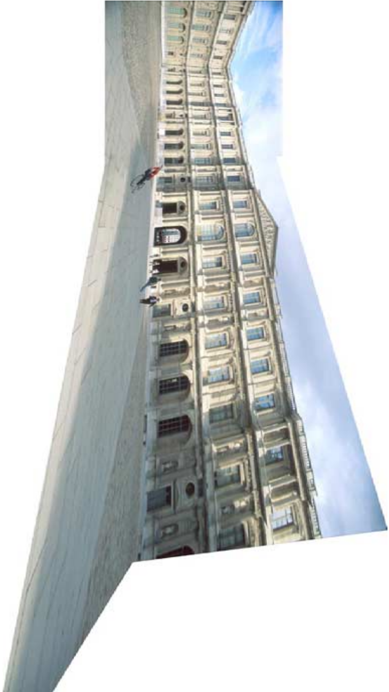
Figure 3.5: Mosaic formed of two pictures. The mosaic has been warped according to two planes, identified by the multi-planar model. The algorithm kept the texture of the plane closest to the camera. This allows to warp the part of the image that does not contain any stereo information. The apparent distortion of the figure is due to the large viewing angle. The original images were taken with a 24mm lens.
