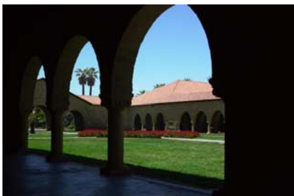
Figure 6.1: Image of a high dynamic range scene captured and rendered with traditional techniques. The details under the arches are totally lost whereas the observer who took the picture was able to see them.
