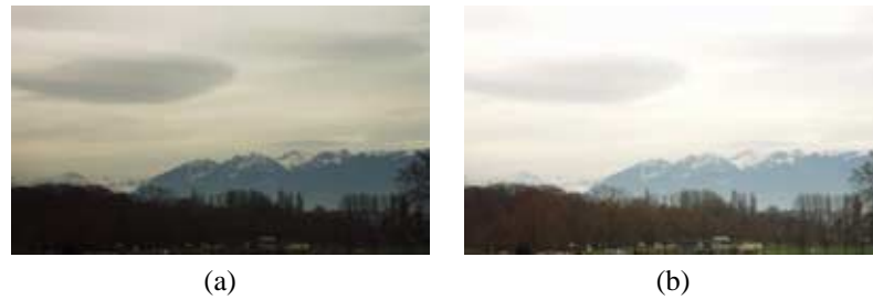
Figure 5.9: Images used to fit a polynomial OECF model of the camera. The images have the same white point but different exposures.
