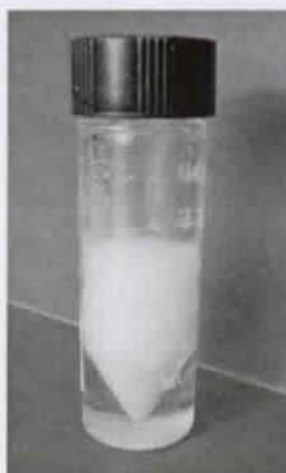
Fig. 5.23: Picture of a typical sol obtained with HCl at \text{pH} > 4.2 . Picture taken after 4 h of mixing.
