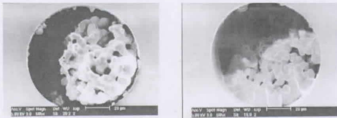
Fig. 7.12: SEM pictures of a macroporous ormosils monoliths made in a capillary (I.D.= 100\ \mu\text{m} ). The two pictures show two cross-sections of the same capillary. The metastable sol used to make this monolith is analogous to the one used for Fig. 7.11. (SEM pictures \times 695 , bar scale 20\ \mu\text{m} )
