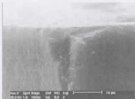
Fig. 7.4: Monolith made with H_r=100\% . (SEM picture \times 1932 , bar scale 5 \mu\text{m} ).
