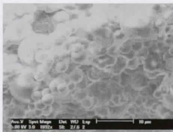
Fig. 7.19: SEM picture of a fracture surface of an ormosil monolith made with glutaronitrile. (SEM picture \times 1932 , bar scale 10 \mu\text{m} )
