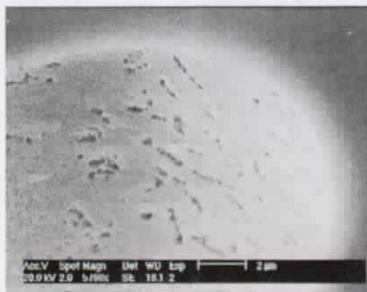
Fig. 3.13: Porous silica layer at the surface of the inner capillary wall. (SEM picture \times 5798 , bar scale: 2 \mu\text{m} )
