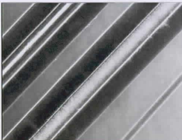
Fig. 7.14: Monolithic columns for CEC according to the protocol in chapter 7.4 with H_T=200\% .
