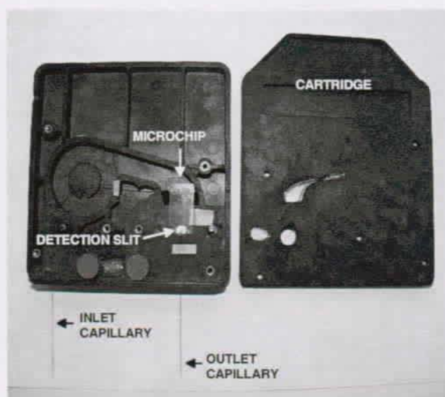
Fig. 9.3: CEC chip housed in the Beckman's cartridge used with the P/ACE 5500 system. The detection slit ( 800 \times 100 \mu\text{m} ) of the cartridge was aligned with the outlet of the chip's separation channel to allow for detection. The cooling system of the cartridge adapted to house a chip was short-circuited to avoid leakage of the cooling liquid.
