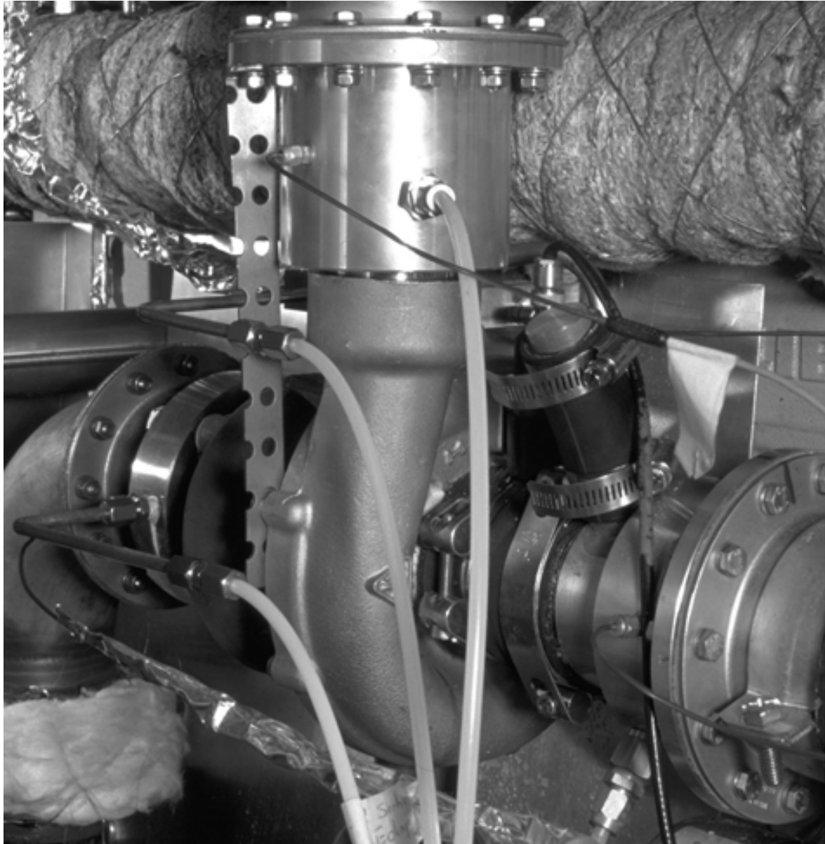
Figure C.7: Turbocharger KKK type K27 instrumented for temperature and pressure measurements at the inlet and outlet of the compressor and turbine.
