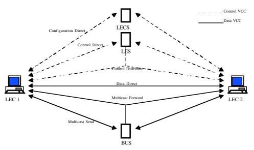
Figure 10: ATM connections for LANE
