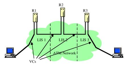
Figure 12: routing for traffic across LIS borders
