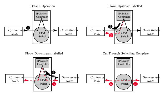
Figure 21: From default routing to cut-through ATM connection
