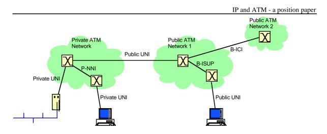
Figure 8: ATM network architecture and interfaces
