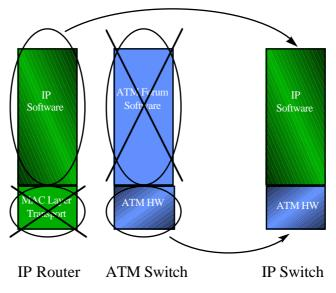
Figure 20: IP Switching concept
