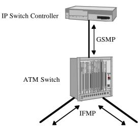
Figure 19: IP Switching Architecture
