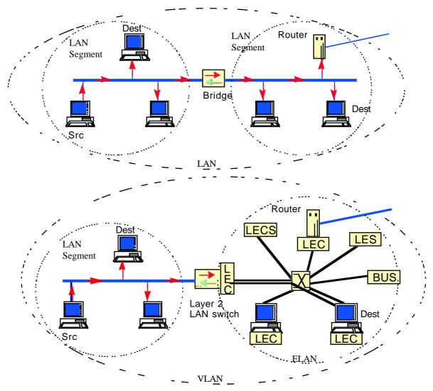
Figure 9: Classical LAN and Emulated LAN architecture
