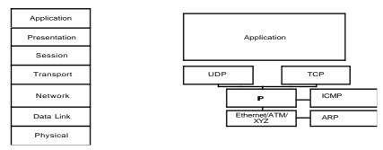
Figure 1: IP in the Protocol Stack
