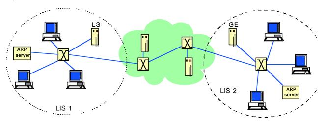
Figure 11: Classical IP over ATM network architecture
