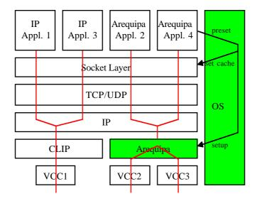
Figure 18: Arequipa in the protocol stack
