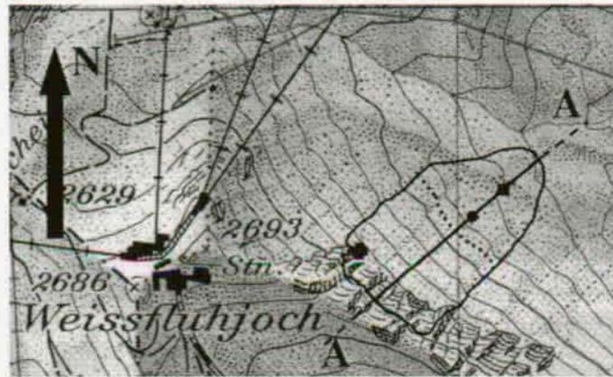
Figure 6.3: Situation of profiles in the Meierhoftälli avalanche. Cross: situation of fracture profile (see Figure 6.6). Circle: profile in flat region of runout zone. Square: profile in accumulation zone near moraine wall. The upslope boundary of the depositional area is indicated by a dotted line. Line A-A is the profile line of the terrain profile in Figure 6.4.
