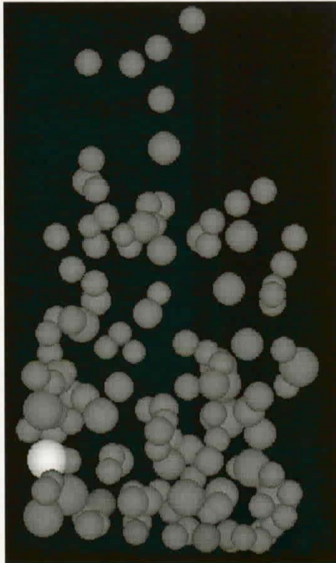
Figure 5.17: An accelerating flow reaches a dilute gas-like state. Picture of model flow after 79 s of running time. Particle material parameters are e=0.8 , b=0.8 , \mu=0.4 .
