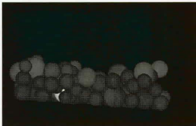
Figure 5.16: Decelerating flow after 2.675 s running time. Particle material parameters are e=0.7 , b=0.4 , \mu=0.6 .
