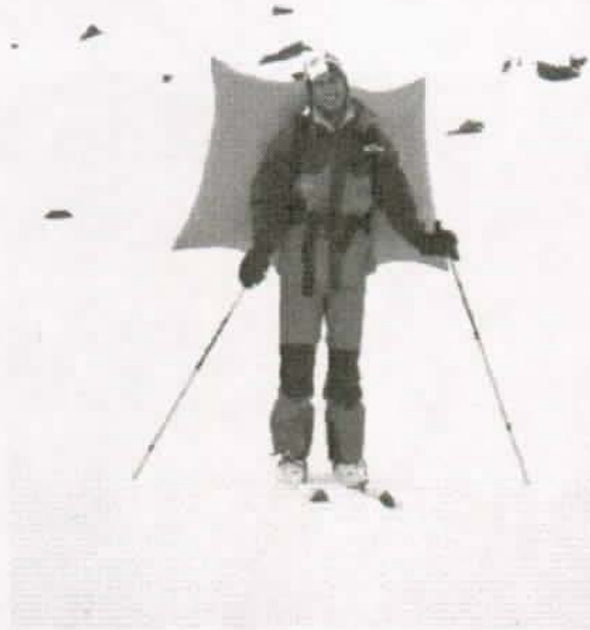
Figure 2.3: Front view of a skier wearing an avalanche balloon backpack with inflated balloons. Photograph by Martin Popp, MPG.
