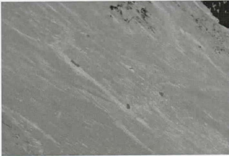
Figure 6.15: Initial position of test bodies after avalanche release. Some bodies were not taken away by the avalanche; they kept lying embedded in a slab-like layer of compressed snow.
