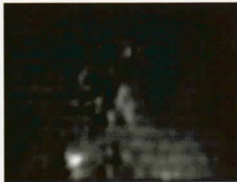
Figure 3.25: CTEM image simulation of a cascade induced by a 10 keV PKA after 30.0 ps (weak coupling), inside a matrix of Al 44 \times 44 \times 44 unit cells (original box) cut and tilted to [015] ZA in WBDF \vec{g}(3.1\vec{g}) , \vec{g} = (200) condition.
