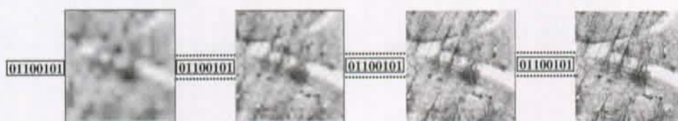
Figure 1.5: Refinement of an aerial photography: Initially a coarse approximation is obtained using a few transform coefficients. Then, the approximation is gradually refined (right to left).
