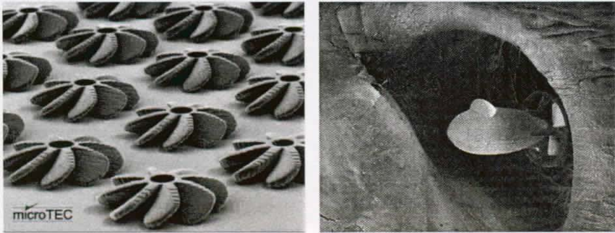
Figure 2-6 On the left: impellers for flow sensors of roughly 600\ \mu\text{m} in diameter. On the right: artist's impression of a micro-submarine in an artery (from [GOT99]). Whereas the flow sensors built with those impellers could prove effective under certain flow configurations, we have great concern on the propulsive capabilities of the micro-submarine.
