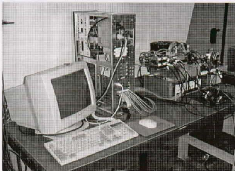
Figure 4.48: Experimental system for the DC-DC converter
