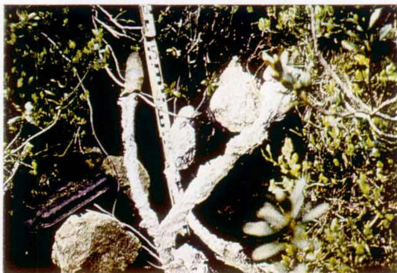
Figure 2. Lysimeter device covered with aluminium and temperature sensors
