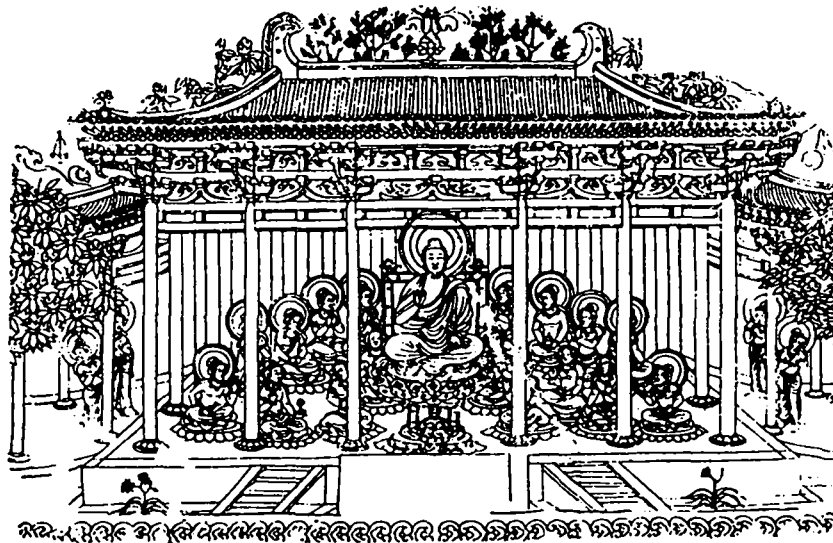
Fig. 495: Carving of an image hall with flying rafters on the lintel of the Dayan-ta 大雁塔 대안탑 of Cien-si 慈恩寺 자은사 (701 - 704 AD, no scale) (after: LIU Dunzhen 劉敦楨 유돈정 (1980), p. 119)
