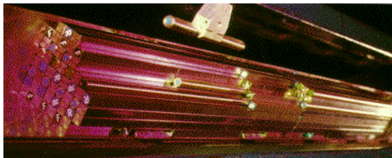
Figure 2-5: Charging of a MASURCA tube using fissile (rectangular) and non-fissile (square) rodlets of 1.27 cm x 1.27 cm lateral dimensions.
