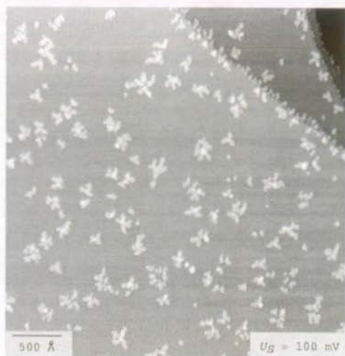
Figure 6.1: Submonolayer growth of Ni on Ag(111) at 130 K. The image has been taken at 77 K.
