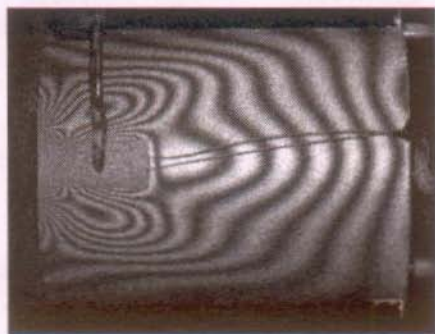
Figure 2-5. Holographic interferometry fringes showing out-of-plane deformation due to thermal loading of a cylinder made of Invar.
