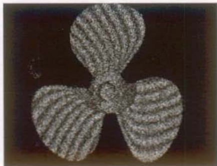
Figure 2-12. Contouring fringes obtained on a miniature propeller.
