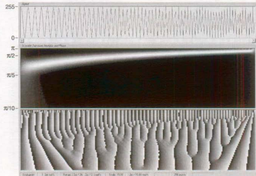
Figure 6-4. Morlet wavelet transform of a linear chirp, presented as a scalogram. The vertical scale goes from \pi/10 to \pi rad/s.
