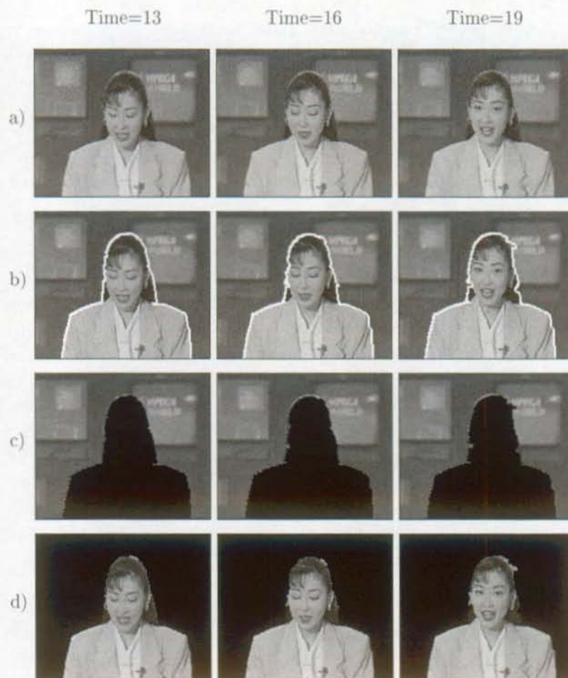
Figure 6.10: "Akiyo": Spatio-temporal segmentation and object tracking. (a) Frames at time 13, 16 and 19, (b) spatio-temporal segmentation at time 13, 16 and 19, (c) object "background" at time 13, 16 and 19, (d) object "woman" at time 13, 16 and 19.
