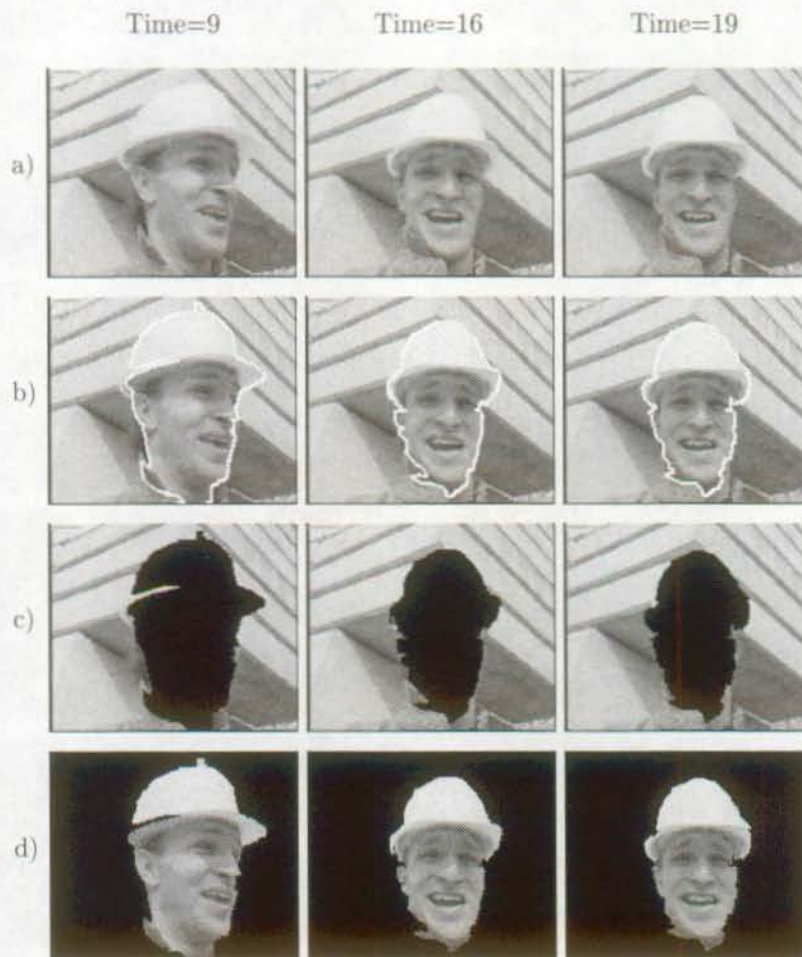
Figure 6.14: "Foreman": Spatio-temporal segmentation and object tracking. (a) Frames at time 9, 16 and 19, (b) spatio-temporal segmentation at time 9, 16 and 19, (c) object "background" at time 9, 16 and 19, (d) object "man" at time 9, 16 and 19.
