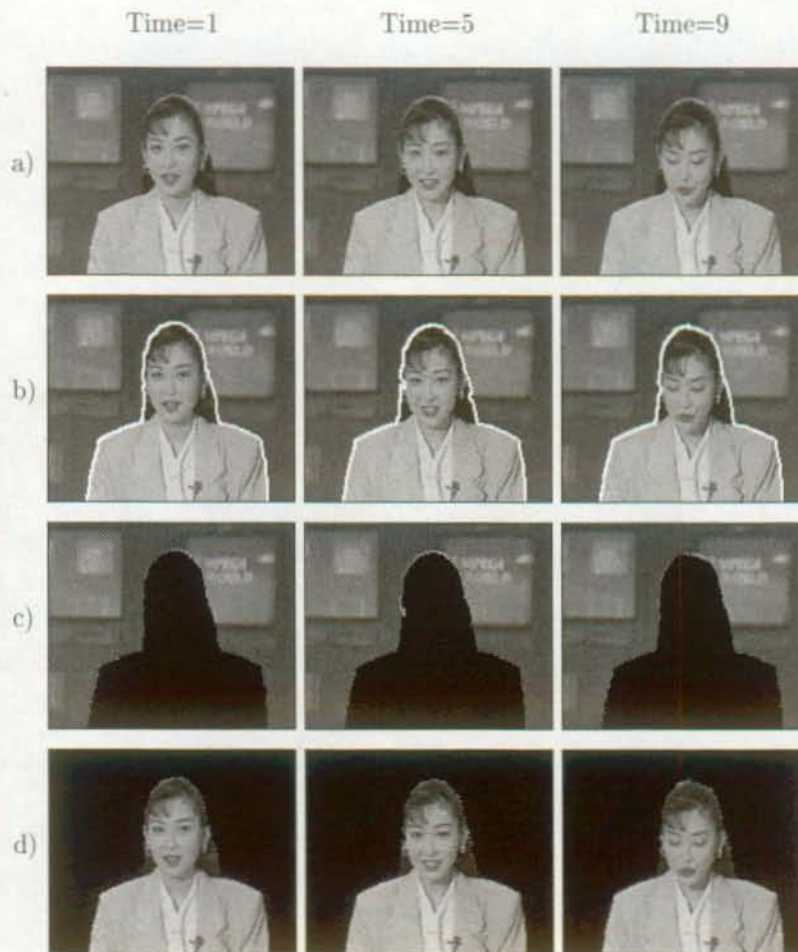
Figure 6.9: "Akiyo": Spatio-temporal segmentation and object tracking. (a) Frames at time 1, 5 and 9, (b) spatio-temporal segmentation at time 1, 5 and 9, (c) object "background" at time 1, 5 and 9, (d) object "woman" at time 1, 5 and 9.
