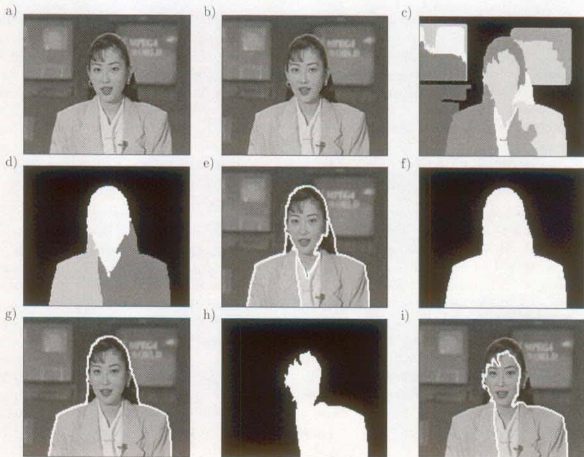
Figure 5.11: “Akiyo”: Spatio-temporal segmentation using arbitrarily shaped initial regions. (a) Previous frame after global motion compensation, (b) current frame, (c) set of initial regions, (d) spatio-temporal segmentation after having applied the strong rule, (e) boundaries of the spatio-temporal segmentation after having applied the strong rule superimposed onto the current frame, (f) spatio-temporal segmentation after having applied both rules, (g) boundaries of the spatio-temporal segmentation after having applied both rules superimposed onto the current frame, (h) spatio-temporal segmentation obtained with the technique proposed by Dufaux et al. , (i) boundaries of the spatio-temporal segmentation obtained with the technique proposed by Dufaux et al. superimposed onto the current frame.
