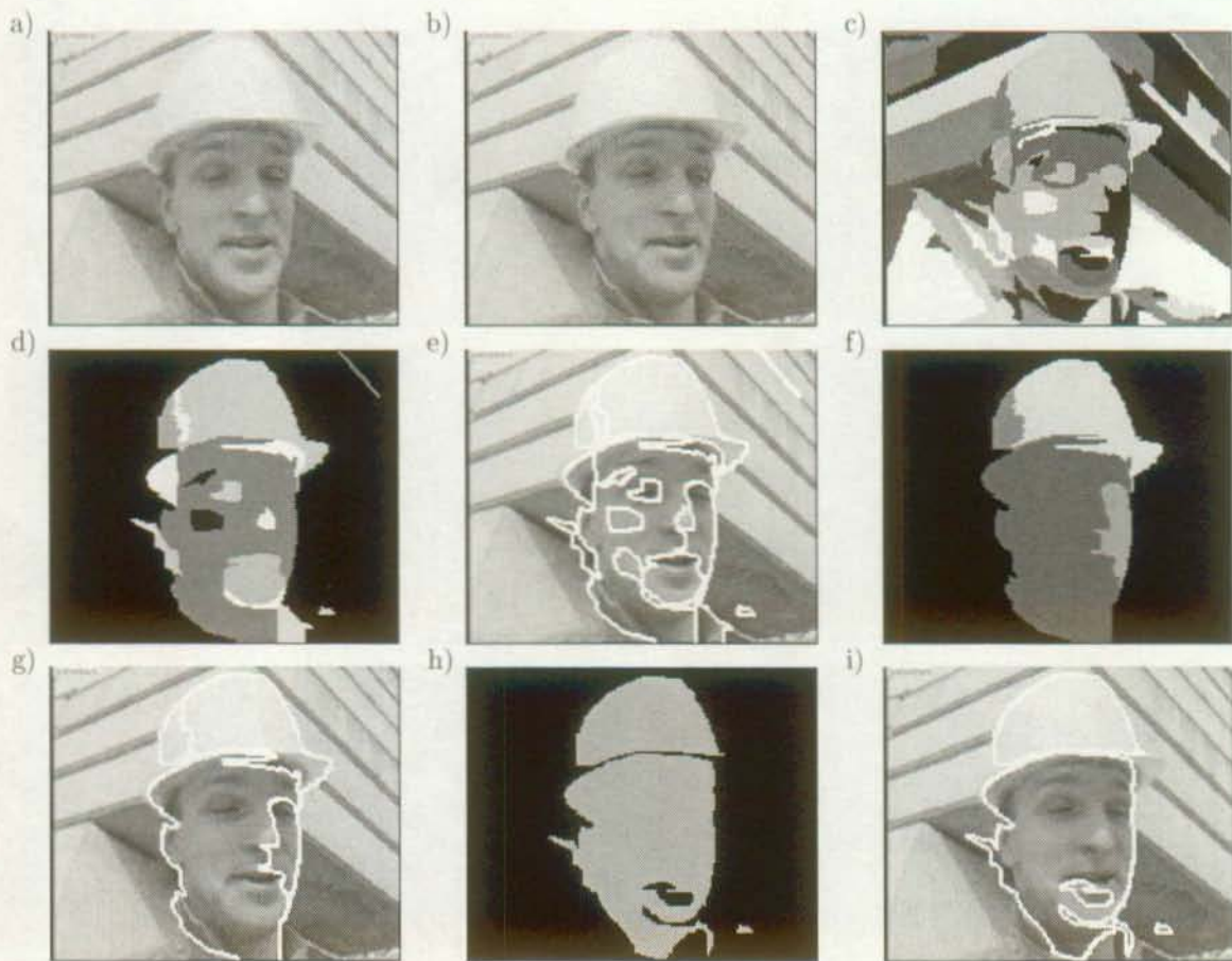
Figure 5.13: "Foreman": Spatio-temporal segmentation using arbitrarily shaped initial regions. (a) Previous frame after global motion compensation, (b) current frame, (c) set of initial regions, (d) spatio-temporal segmentation after having applied the strong rule, (e) boundaries of the spatio-temporal segmentation after having applied the strong rule superimposed onto the current frame, (f) spatio-temporal segmentation after having applied both rules, (g) boundaries of the spatio-temporal segmentation after having applied both rules superimposed onto the current frame, (h) spatio-temporal segmentation obtained with the technique proposed by Dufaux et al. , (i) boundaries of the spatio-temporal segmentation obtained with the technique proposed by Dufaux et al. superimposed onto the current frame.
