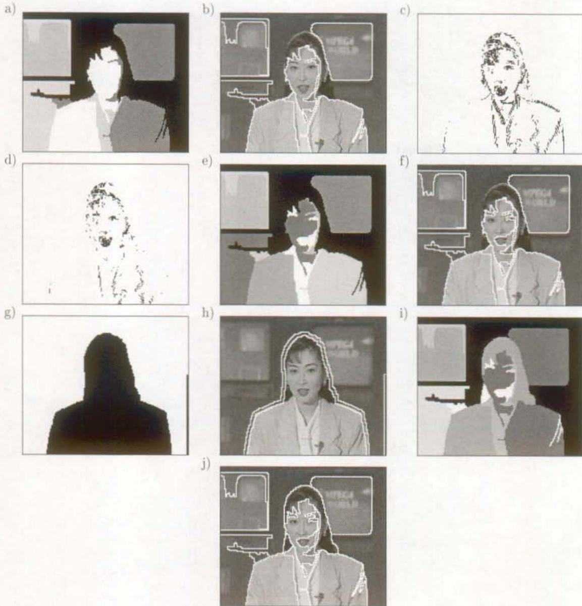
Figure 4.8: "Akiyo": Definition of spatio-temporally homogeneous regions. (a) Set of regions \mathcal{R} after the spatial segmentation, (b) boundaries of the set of regions \mathcal{R} obtained after the spatial segmentation superimposed onto the current frame, (c) DFD before correcting for the disocclusion effects, (d) DFD after correcting for the disocclusion effects, (e) set of regions \mathcal{R} after the use of temporal information, (f) boundaries of the set of regions \mathcal{R} obtained after the use of temporal information superimposed onto the current frame, (g) change detection mask, (h) border areas of the change detection mask are shown onto the current frame, (i) final set of regions \mathcal{R} after the use of change information, (j) boundaries of the final set of regions \mathcal{R} obtained after the use of change information superimposed onto the current frame.
