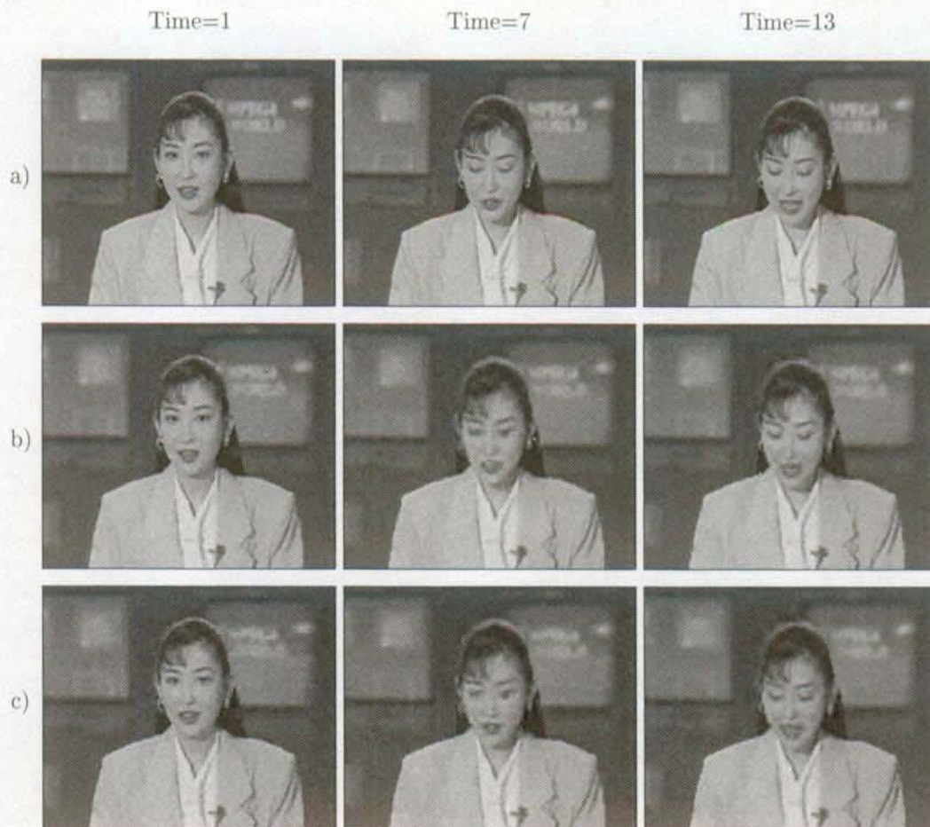
Figure 7.11: "Akiyo": Coding results at different bitrates for the proposed video coding scheme. (a) Original frames at time 1, 7 and 13, (b) sequence coded at 25 kbits/s, (c) sequence coded at 19 kbits/s.
