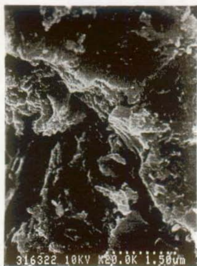
Figure 16: SEM photograph with magnified view (x 20'000) of "fractal" TiO 2 ceramic electrode made by controlled hydrolysis of a TiCl 4 solution.
