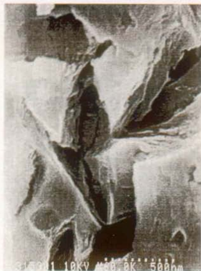
Figure 17: SEM photograph with the magnified view ( \times 60'000 ) of the fractal \text{TiO}_2 ceramic material.
